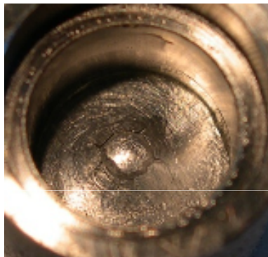
radial cracks also appear at the bottom side
