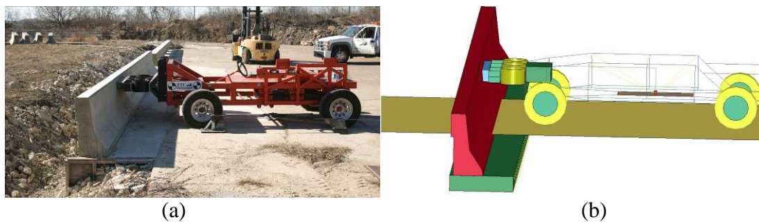
Figure 4 Bogie impact setup for the T501 safety shape rail (a) test, (b) model.
