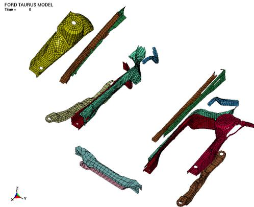
Figure 3: Exploded view of structural components influenced by design variables.
