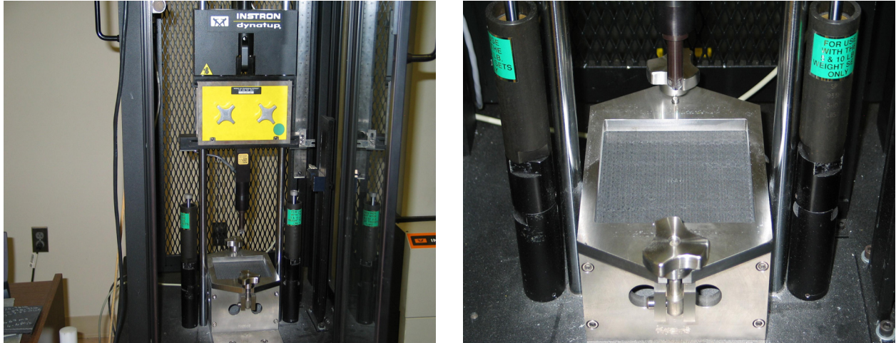
(a) Drop tower and impactor
