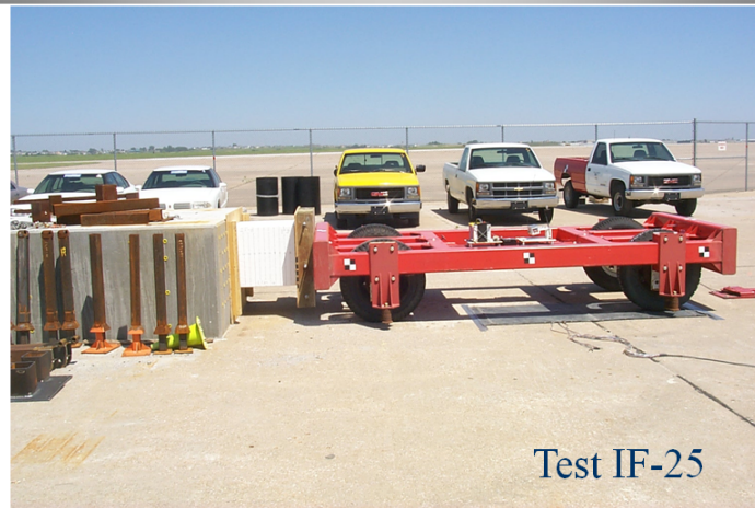
Figure 2. Typical Bogie Testing Set-up
