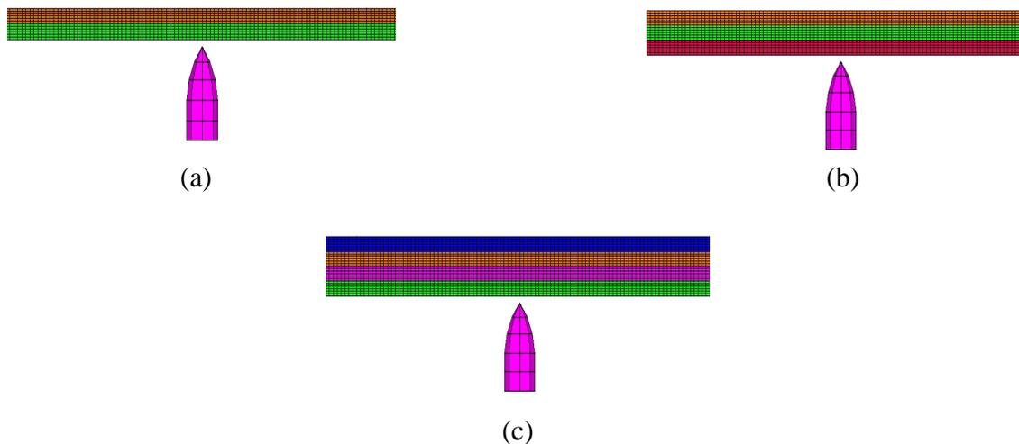
Fig. 9. Sectional views of finite element models of multi-layered MS plates and projectiles modeled with solid elements: (a) double-layered, (b) triple-layered, and (c) quadruple-layered
