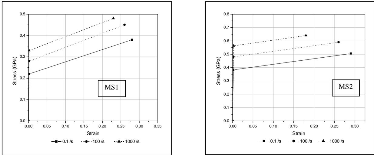
Fig. 3. True stress vs. true strain behaviors at different strain rates for MS1 and MS2 targets adapted from [22]
