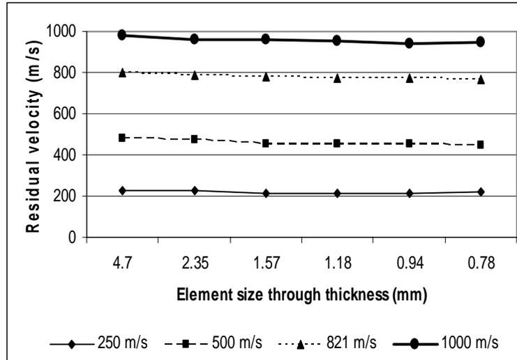
Fig. 8. Effect of projectile impact velocity on convergence of computed residual velocities for a 4.7 mm thick MS1 plate modeled with solid elements
