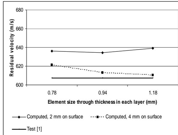
Fig.12. Projectile residual velocities for impact on quadruple-layered MS1 plates of equal thickness of 4.7 mm depth
