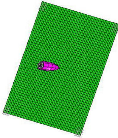
Fig.1. Plate modeled with shell elements
