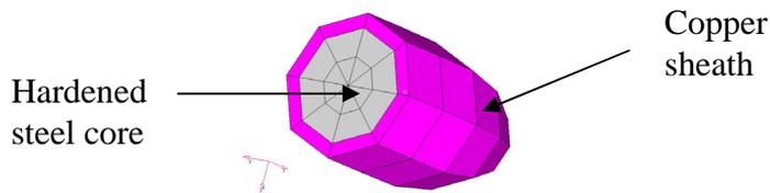
Fig.2. Modeling of jacketed projectile with solid elements
