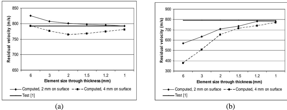
Fig. 7. Projectile residual velocities for impact on MS2 plates of 6.0 mm depths is modeled using shell elements (impact velocity: 866.3 m/s) with (a) CESS interface; (b) CAG interface
