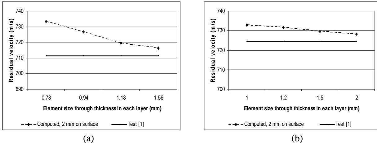
Fig.10. Projectile residual velocities for impact on double-layered plates of equal thickness: (a) MS1 plates of 4.7 mm layer depth; (b) MS2 plates of 6 mm layer depth
