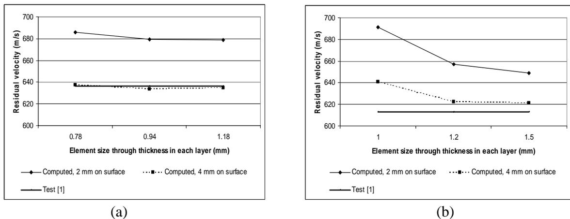
Fig.11. Projectile residual velocities for impact on triple-layered plates of equal thickness: (a) MS1 plates of 4.7 mm layer depth; (b) MS2 plates of 6 mm layer depth
