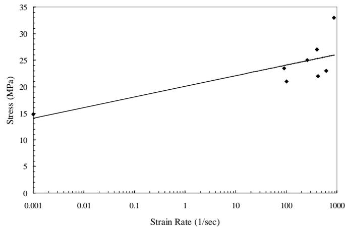
Figure 3. Strain rate sensitivity for single crystal ice.
