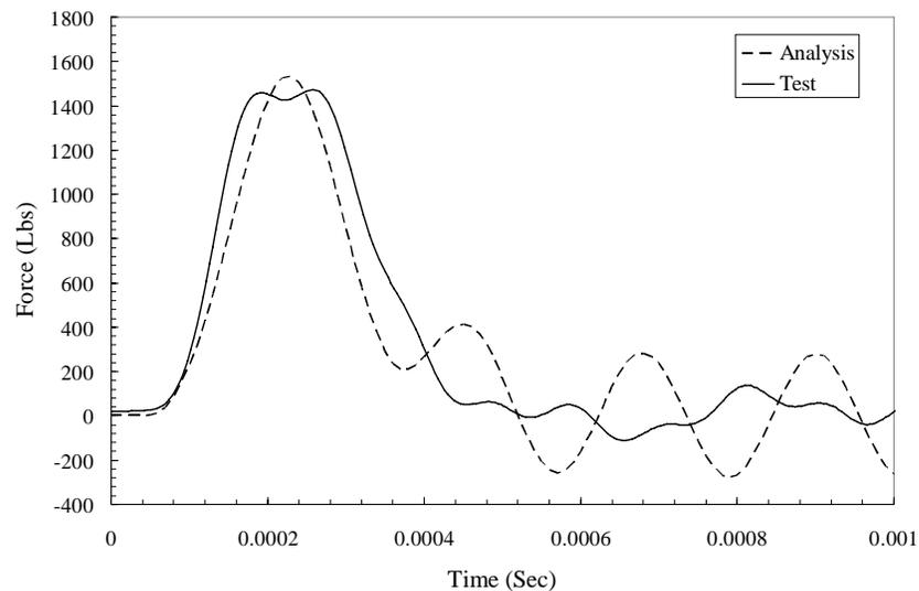
Figure 15. Test analysis comparison at 700 ft/sec, 45° setup.
