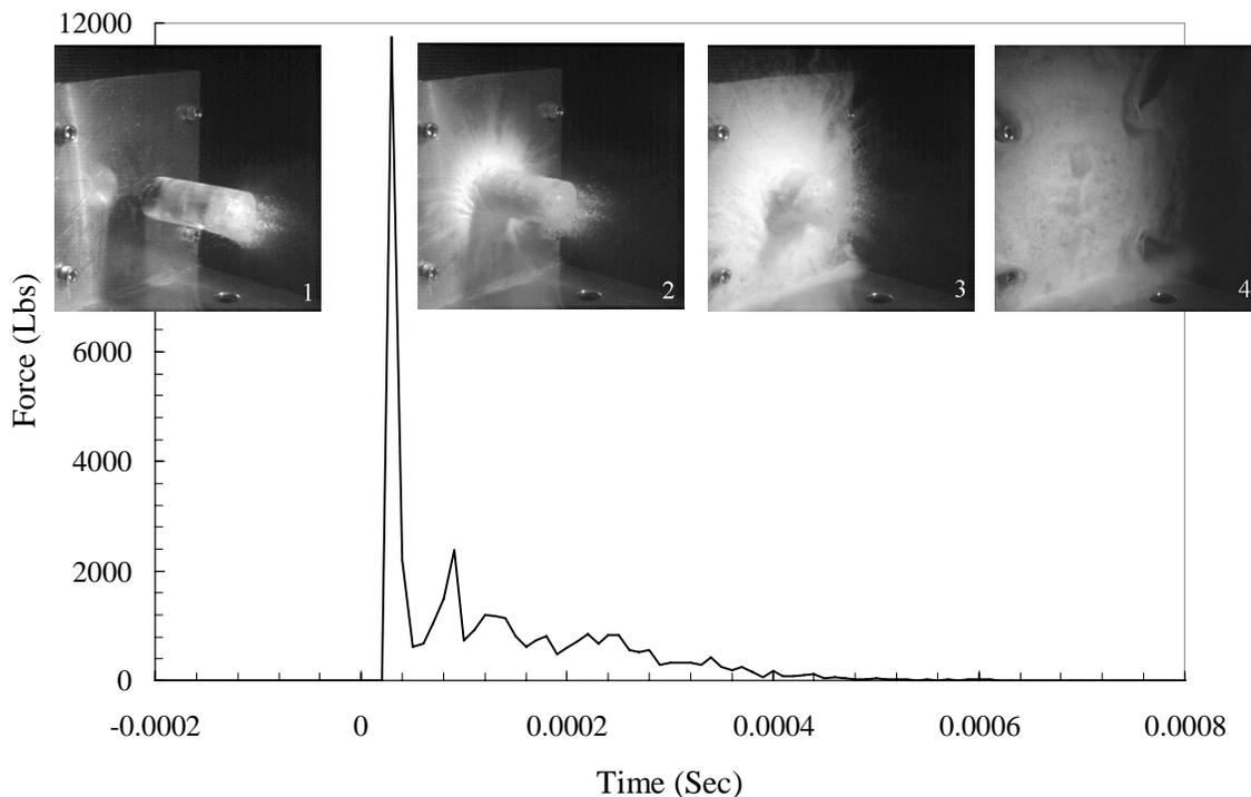
Figure 13. Computed contact force at 500 ft/sec, with high speed images of a ballistic test.
