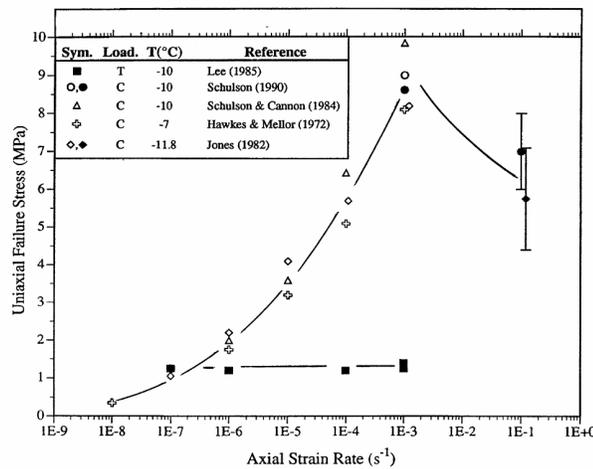
Figure 2. Flow stress as a function of strain rate, reprinted from [7].
