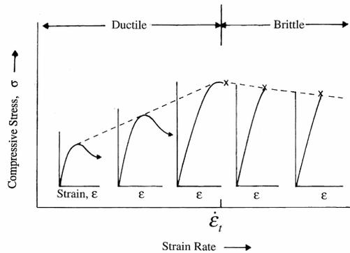
Figure 1. Modes of failure in ice as a function of strain rate, reprinted from [7].
