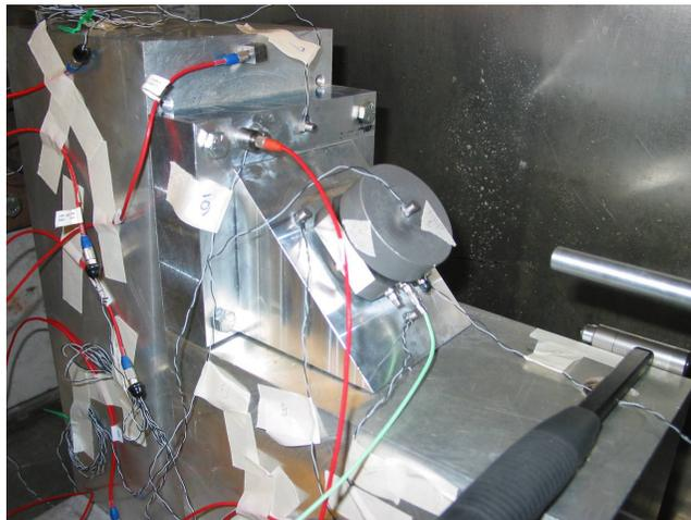
Figure 9. Target plate in the 45° configuration with modal survey instrumentation.
