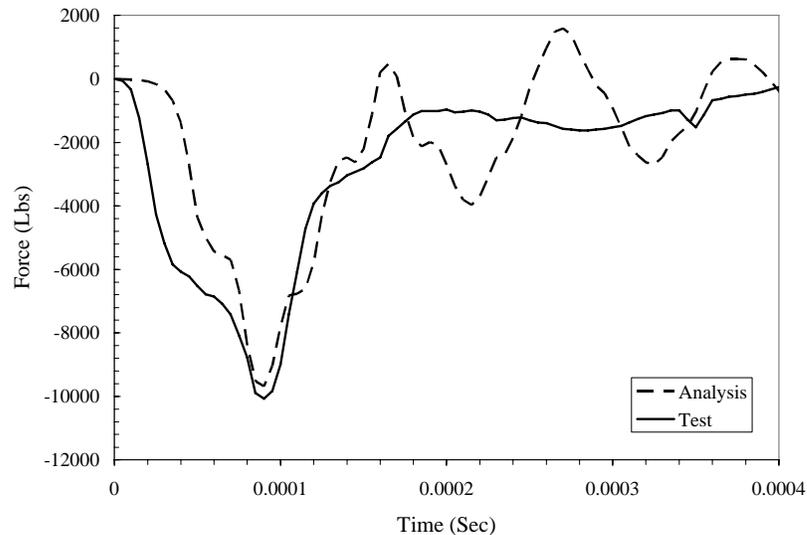
Figure 18. Test analysis comparison of Kim and Kedward Test 54; 1.68" diameter sphere at 413 ft/sec.
