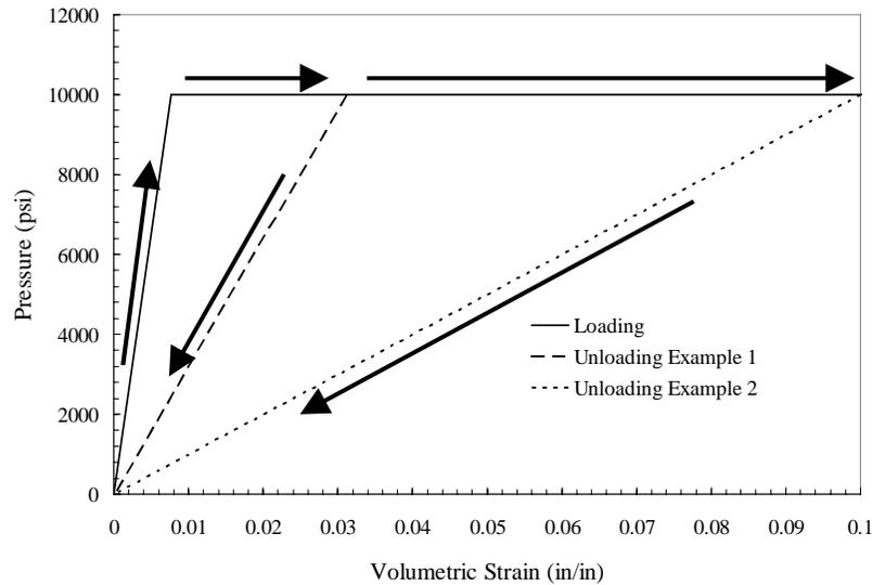
Figure 5. Equation of state with loading and unloading.
