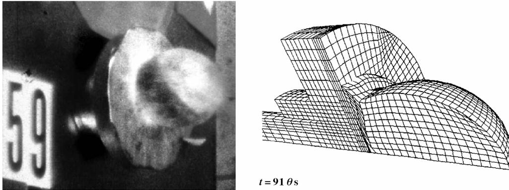
Figure 4. Comparison of an experiment to a calculation of a 42.7 mm diameter ice ball fired at 73.5 m/s at a time of 91  $\mu$ s. Reprinted from [4].
