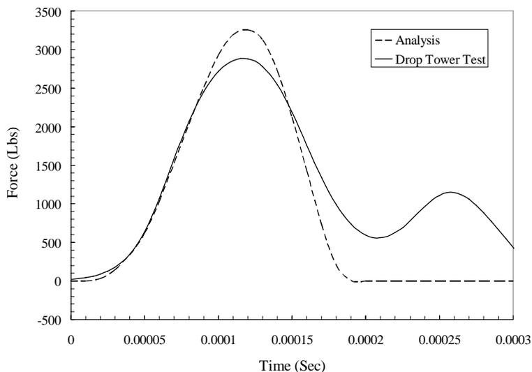
Figure 17. Test analysis comparison from the LaRC drop tower at 100 ft/sec.
