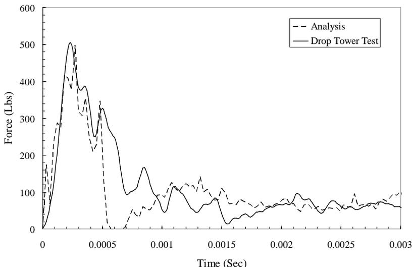
Figure 16. Test analysis comparison from the LaRC drop tower at 20.4 ft/sec.
