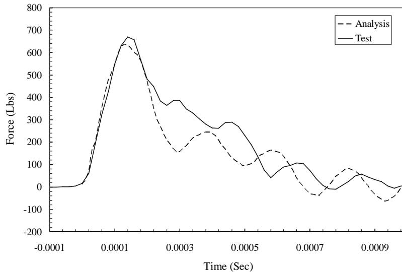
Figure 10. Test analysis comparison at 300 ft/sec, normal orientation.
