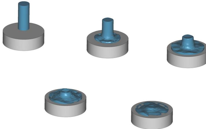
Figure 6. Solid to fluid transition using an Eulerian formulation
