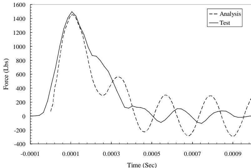
Figure 11. Test analysis comparison at 500 ft/sec, normal orientation.
