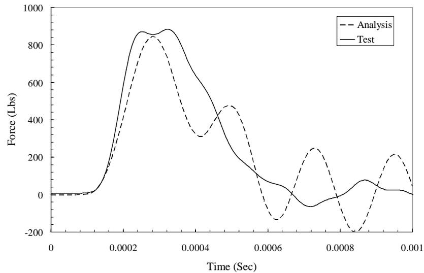
Figure 14. Test analysis comparison at 500 ft/sec, 45° setup.
