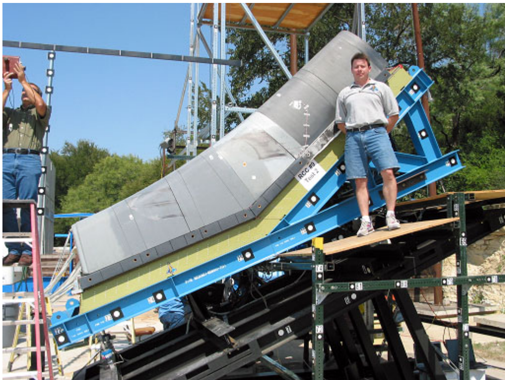
Figure 6. Full-scale Orbiter leading edge test article at Southwest Research Institute ballistic range.
