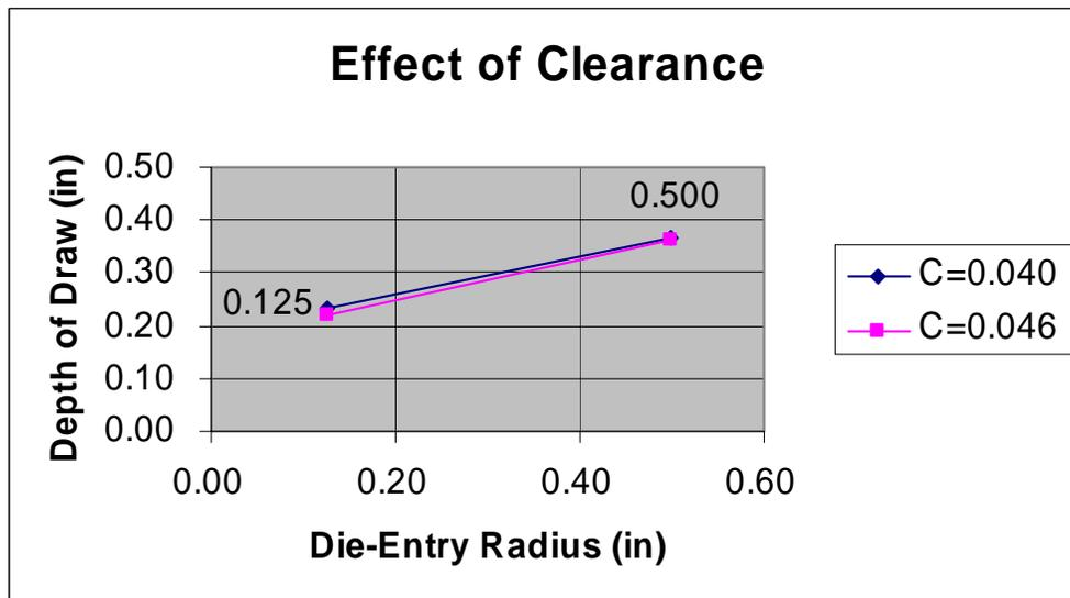
**Figure 8** Influence and interaction of clearance and die-entry radius
