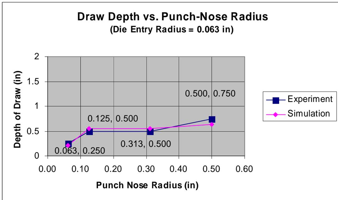
Figure 5 Effect of punch-nose radius on draw depth
