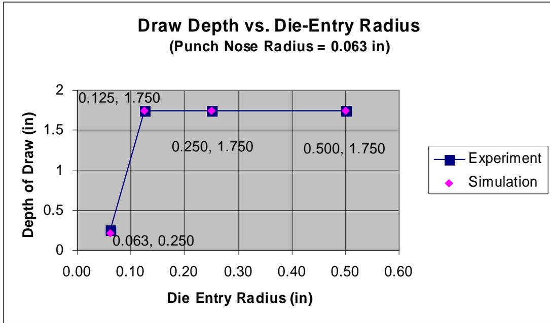
Figure 4 Effect of die-entry radius on draw depth
