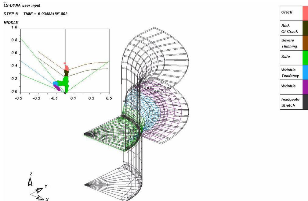
**Figure 11** Forming Limit Diagram (FLD) from a Dynaform<sup>®</sup> simulation with a small number of strain states above the FLD curves
