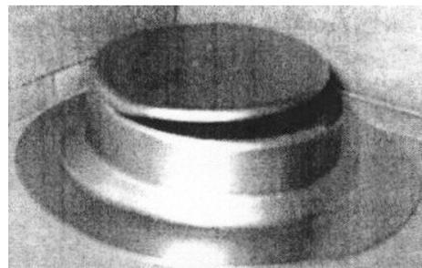
Figure 3 Punch-nose radius failure
