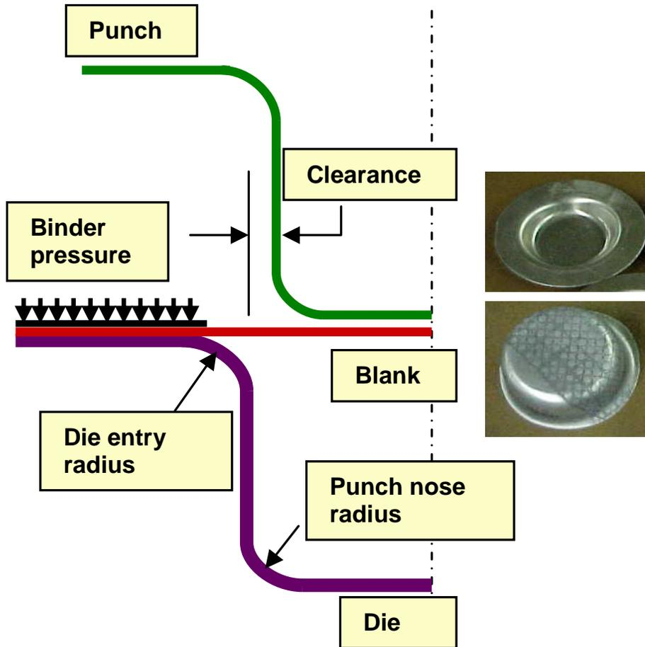
Figure 1 Schematic of the model for stamping design with process parameters
