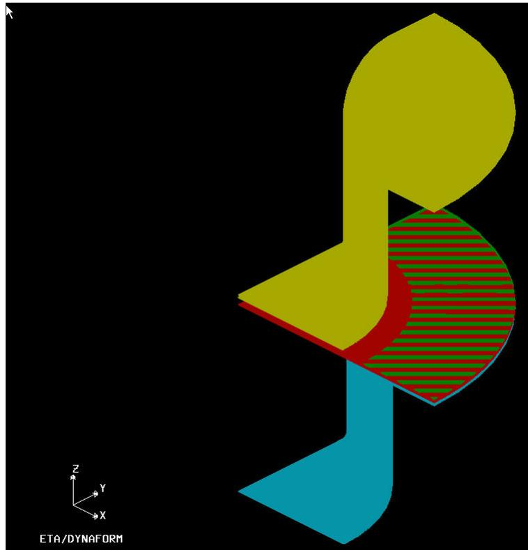
**Figure 6** Model of tools to simulate the drawing of a cylindrical cup
