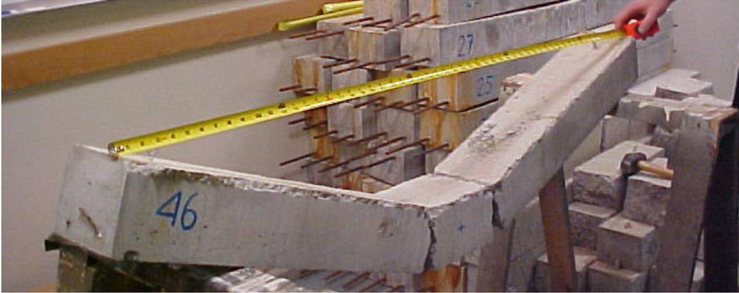
(a) Under-reinforced test specimen.
