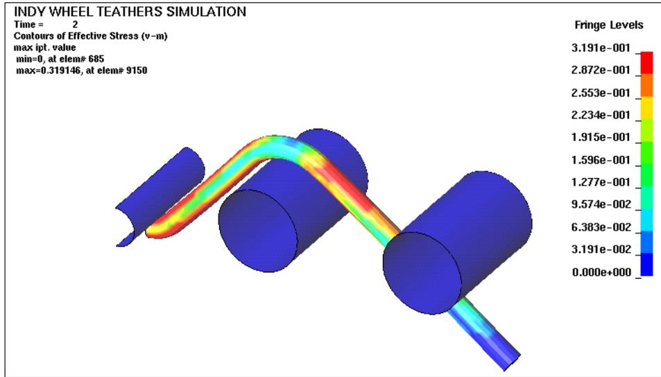
Figure 2. Round Rod between Rollers
