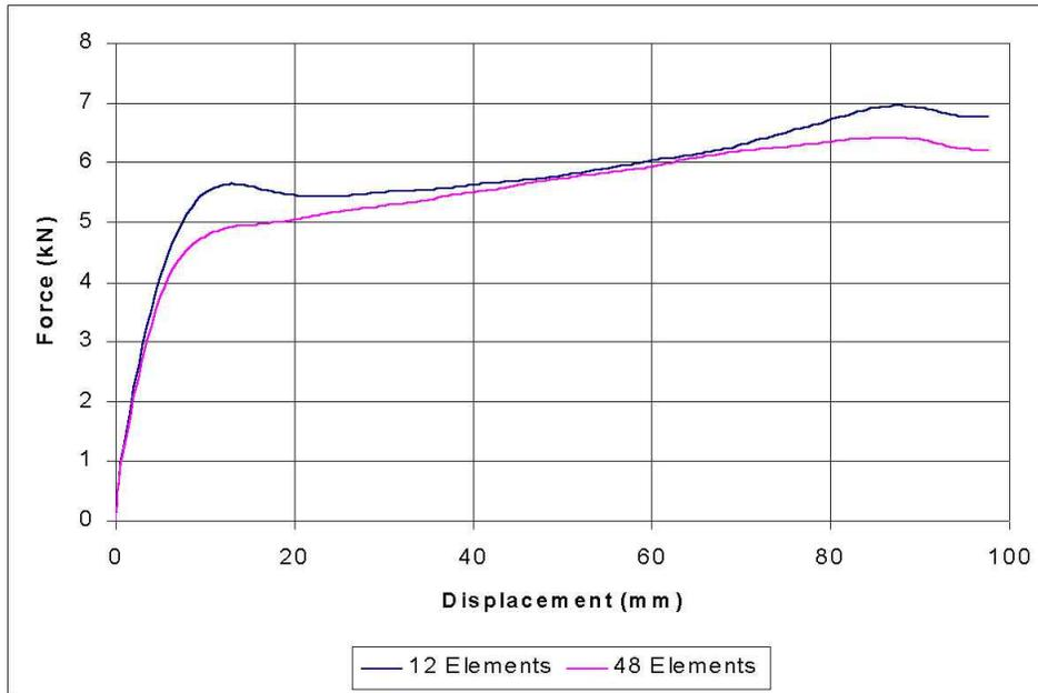
**Figure 5. Comparison between 12 and 48 Elements in the Cross-Section**
