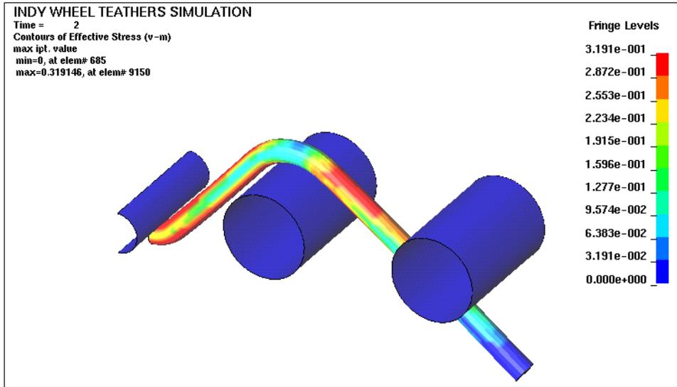
Figure 2. Round Rod between Rollers
