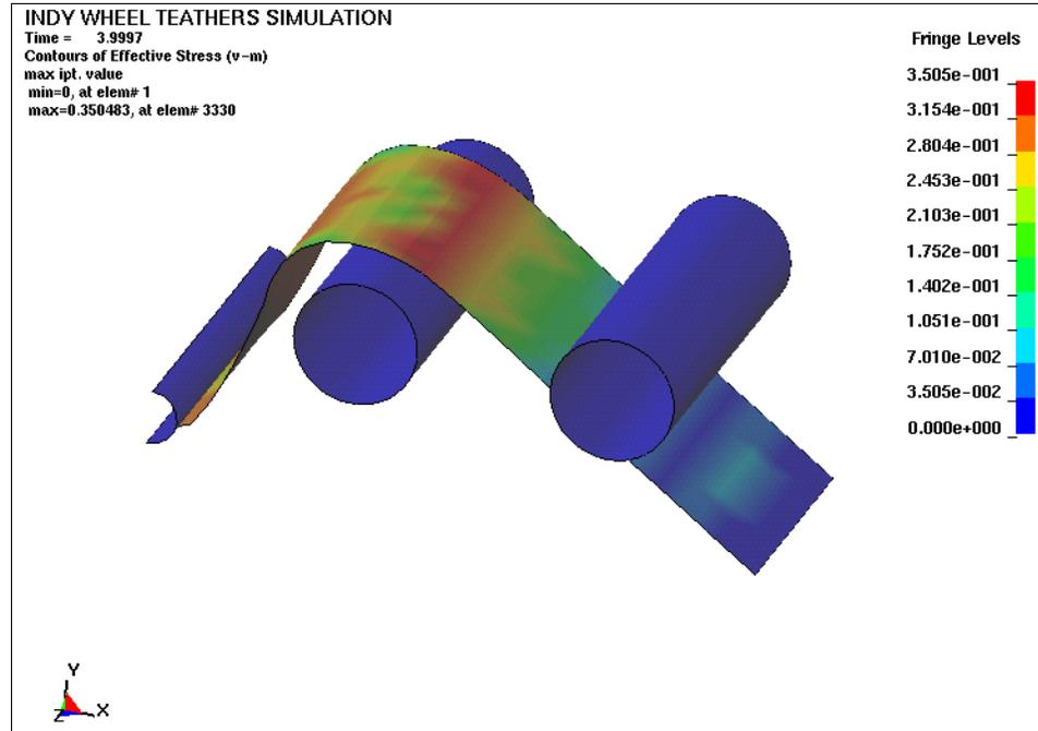
Figure 9. Sheet Steel Section
