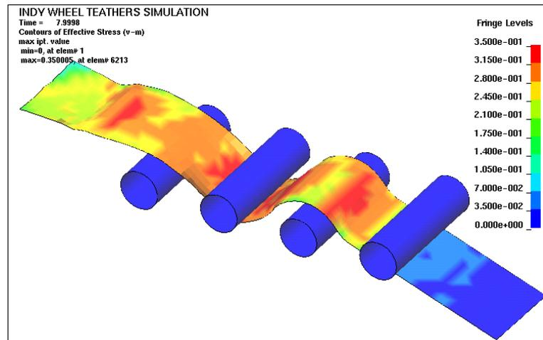
**Figure 12. Sheet Steel Pullout**
