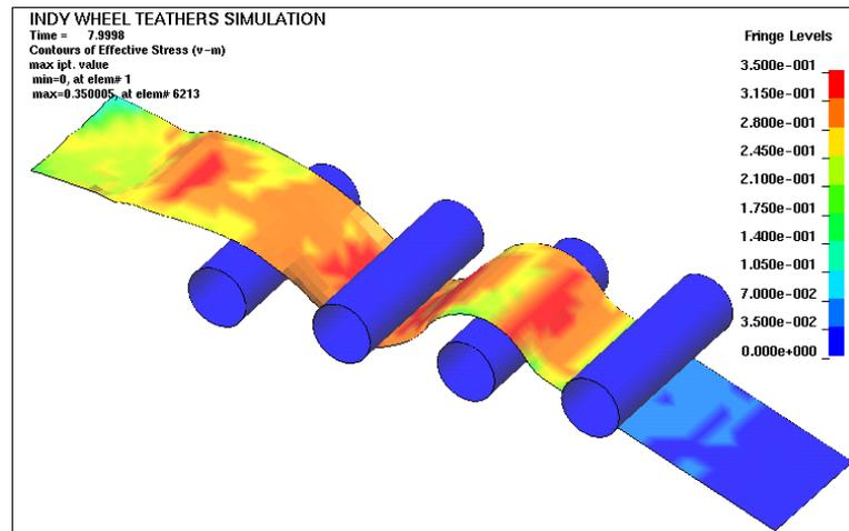
**Figure 12. Sheet Steel Pullout**
