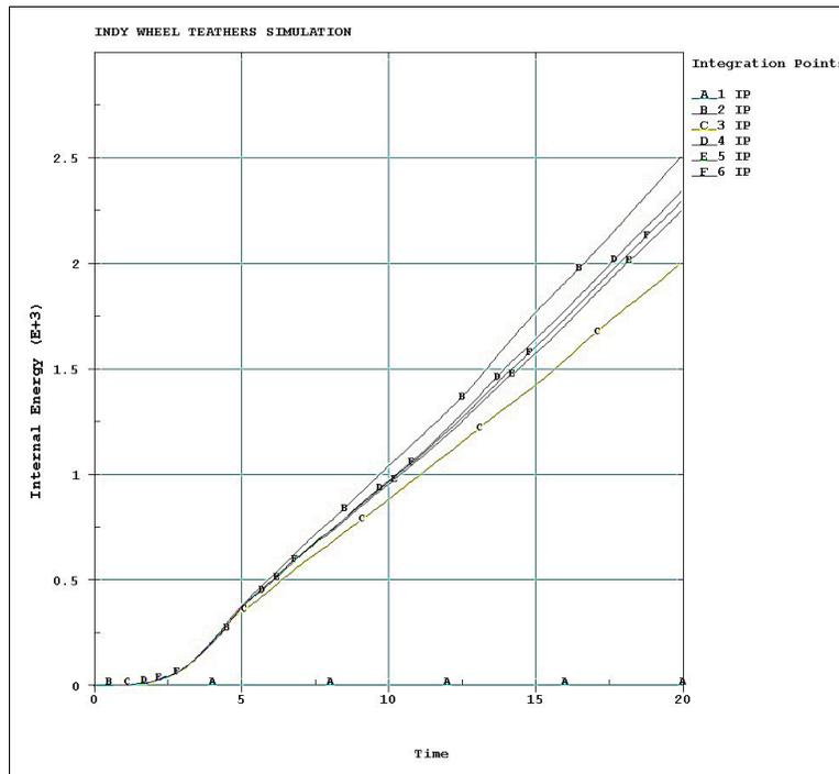
**Figure 11. Effects of Through-the-Thickness Integration Points**
