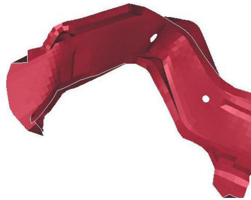
Figure 4. Deformed type-2 rail in Rigid barrier
