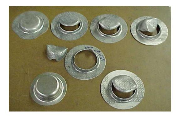
Fig 1: Aluminum cups drawn without any lubricant. Binder force = 6,000 lb approx.
