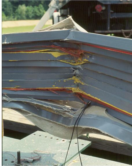
Figure 1. Post Impact Photograph of Multicellular Composite Guardrail Showing “Tearing.”
