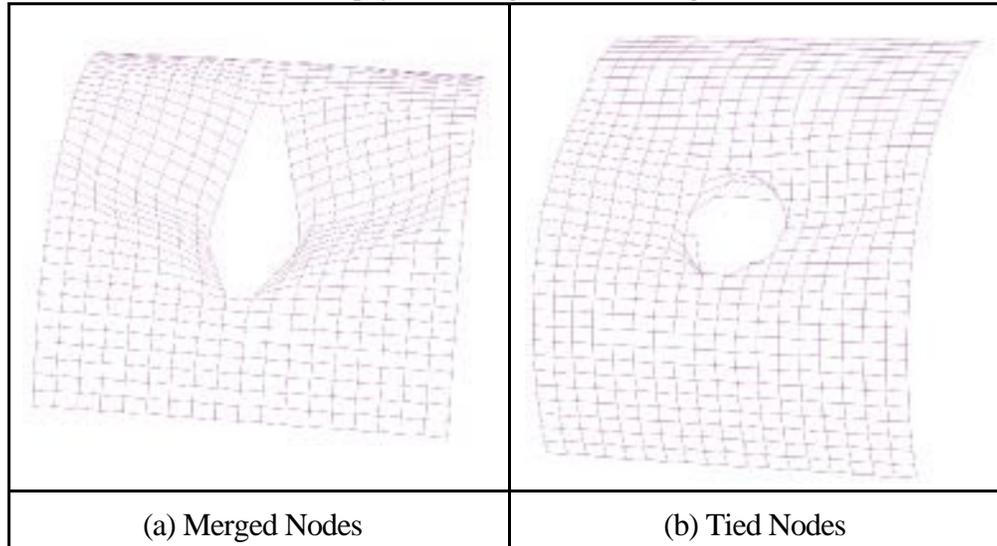
Figure 2. Effects of Tied Nodal Constraints on Failure Mode
