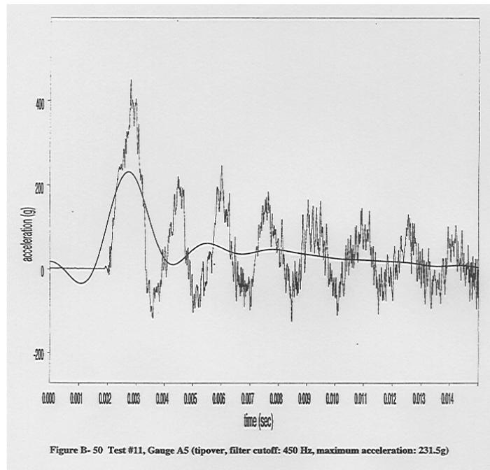
Figure 2. Recorded acceleration from tipover Test #11.
