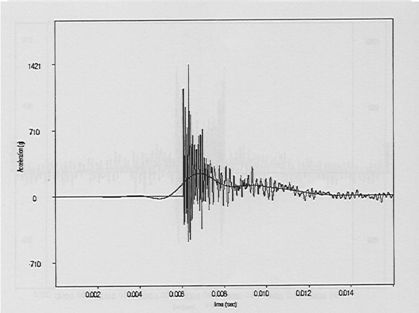
Figure D-5 Finite Element Analysis, Billet (tipover, filter cutoff: 450Hz, max. acceleration: 244.7g)
