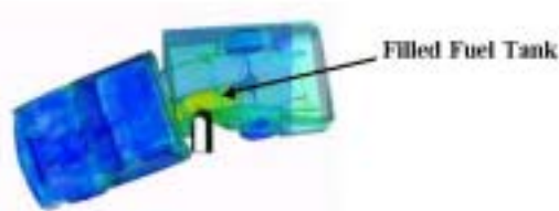
Side Impact With Fuel Oil Inside
