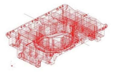
Figure 5. Die Structure IGES Surfaces
