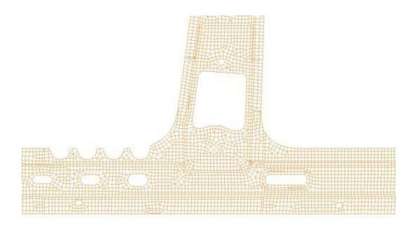
Figure 4: Detail View of Topology Automesher Results of B-Pillar area
