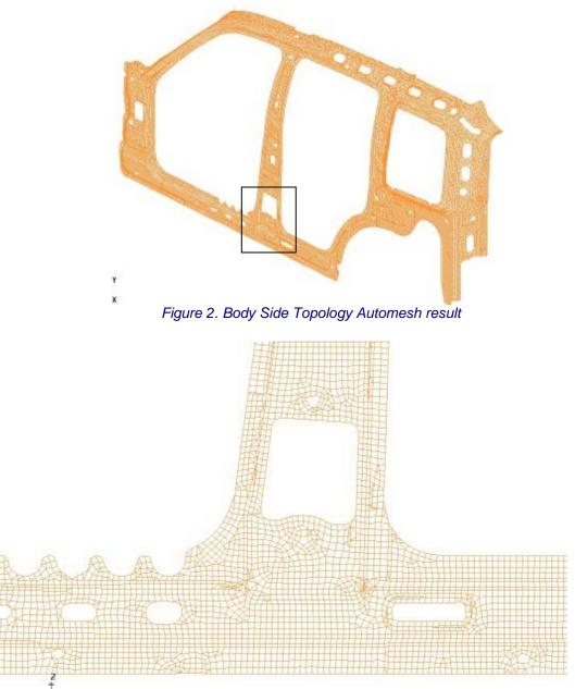
Figure 3 : Detail View of Paving Mesh Results of B-Pillar area
