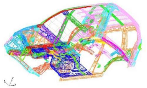
Figure 1. Full BIW CAD Surfaces (102 parts, 20958 Surfaces)
