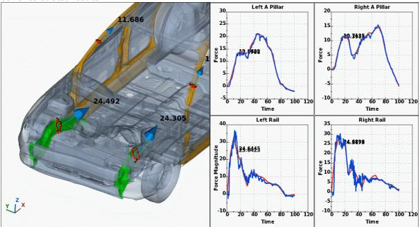
Figure 7. µETA calculated section forces compared to LS-DYNA
