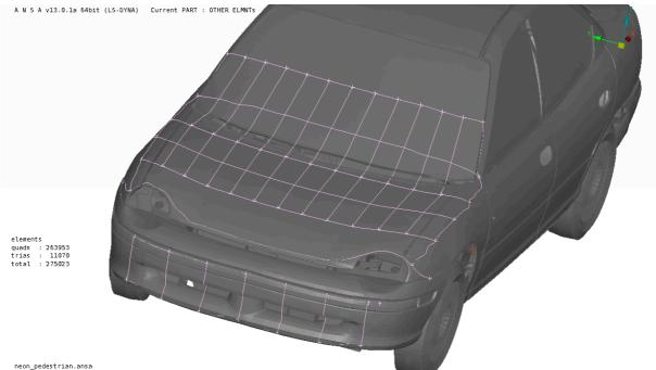
Figure 3. EuroNCAP reference lines automatically created
