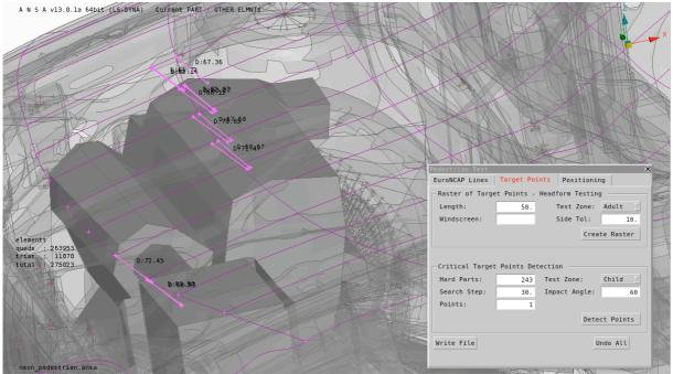
Figure 4. Critical target point detection
