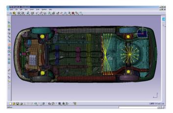
Figure 6: Lumped mass trimming of vehicle.
