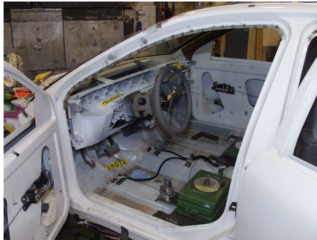
Figure 13- ODB test vehicle after crash and when door was opened with no deformation
