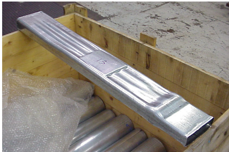
Figure 5-Front portion of the hydroformed rail as manufactured.
