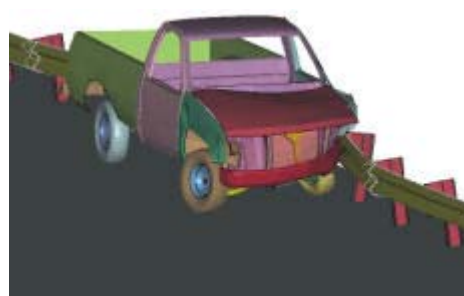
(b) Impact with Steel I-beam post
