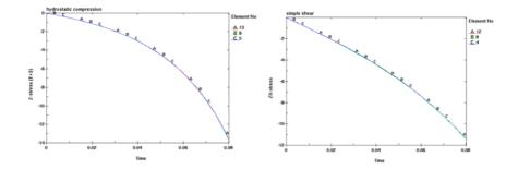
Hydrostatic and shear response of MAT\_181 are equivalent to the Ogden model
