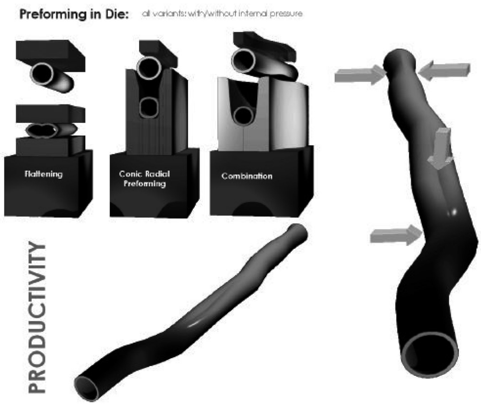
Figure 10: Preforming in Die: Selected Process Variants – Fictitious Component
