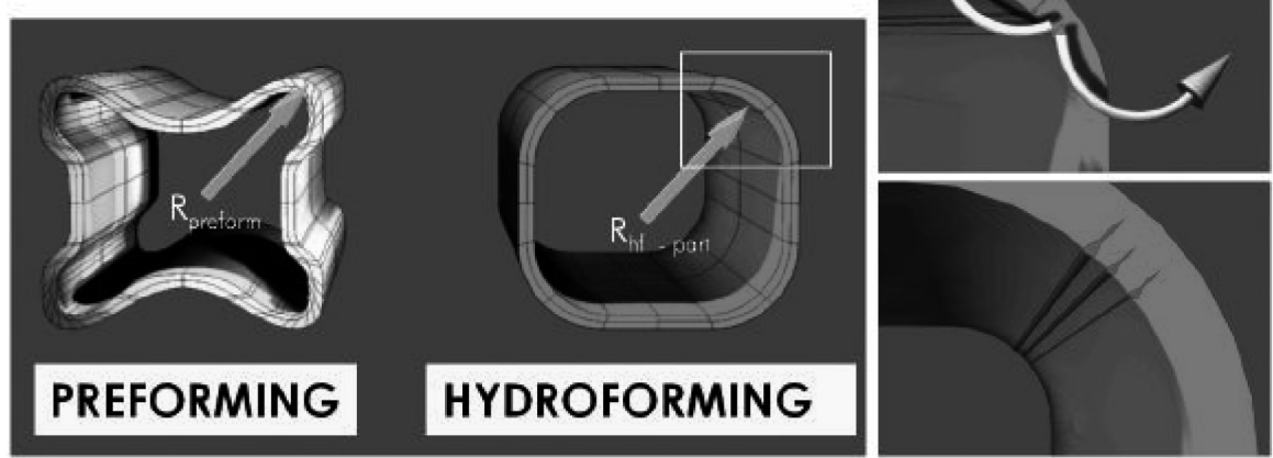
Figure 15: Requirements on Starting Parts for Hydroforming: All Radii after Preforming greater or same as the Final Component Radii
