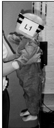
Figure 5 - a view of the dummy used for the experiments. One of the accelerometers can just be made out taped to the forehead of the dummy.
