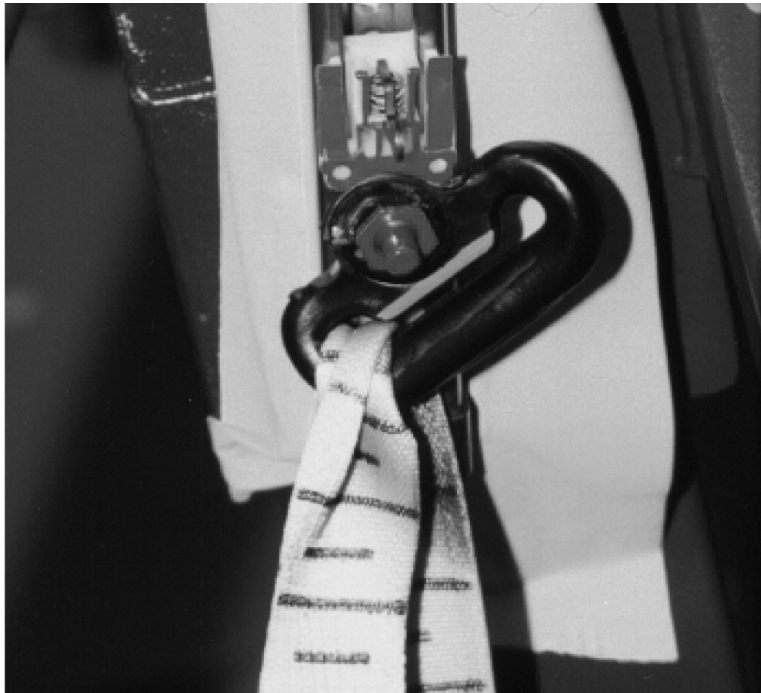
Figure 1b: Example of overturned D-ring
