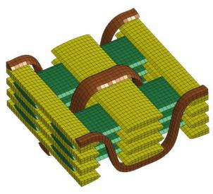
Fig. 3: Finite element model of the RVC.
