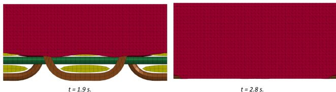
Fig. 6: Resin flow through the RVC.
