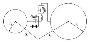
Figure 8 Penalty-based particle-particle interaction in LS-DYNA.
