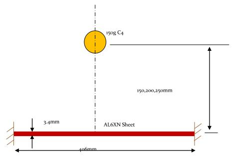
Figure 3 Sketch of the experimental set-up
