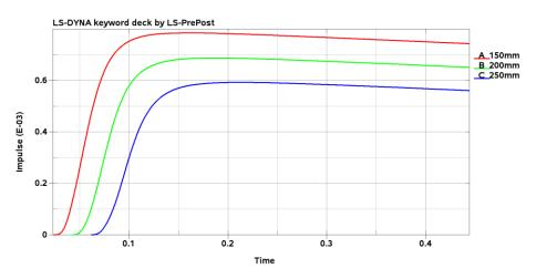
Figure 6 Reflected impulse for 150mm, 200mm and 250mm stand-off distance
