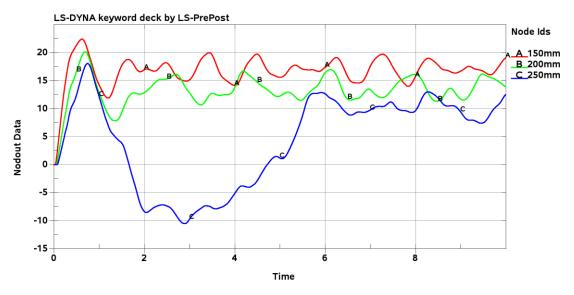
Figure 5 Central node displacement versus time for 150mm, 200mm and 250mm stand-off distance.
