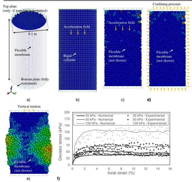
Figure 9 Triaxial compression test model: a) Isometric view of packed sample; b) Sample packing; c) Sustained application of the acceleration field; d) Application of confining pressure; e) Depression of the top plate (displacement field shown); f) Validation against [7]
