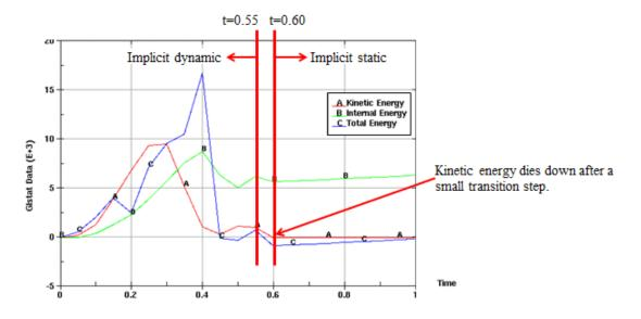
Figure 11. Energy during the switching.
