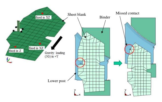
Figure 2. Missed contact between gaging pin and blank edge.
