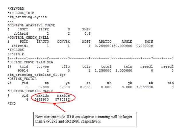
Figure 15. An example of defining starting ID for an adaptive trimming.
