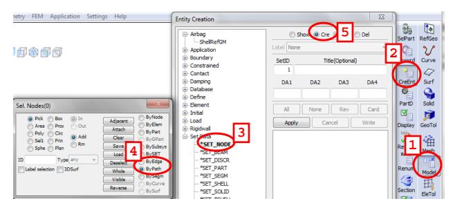
Figure 4. Create a node set "By Path" in LS-PrePost4.0.
