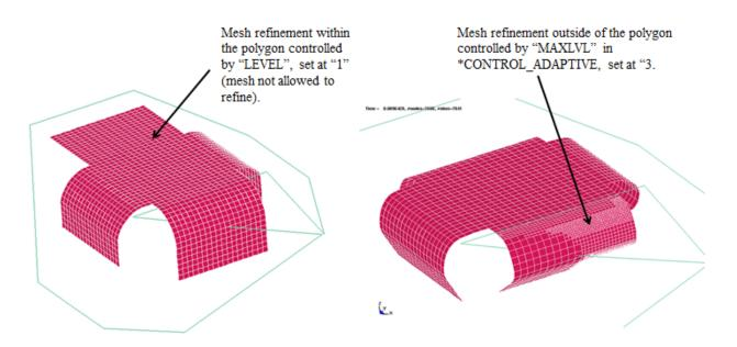
Figure 14. Mesh refinement when defined polygon curve exclude the area of interest, and LEVEL < MAXLVL.
