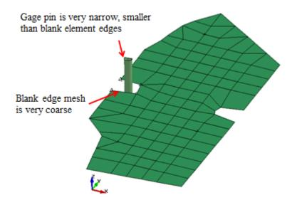
Figure 1. Gaging pin and blank mesh
