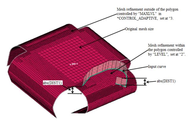
Figure 13. Mesh refinement when defined polygon curve enclose the area of interest, and MAXLVL≠1.
