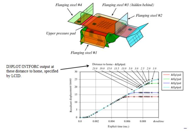
Figure 9. Output control – a flanging example.
