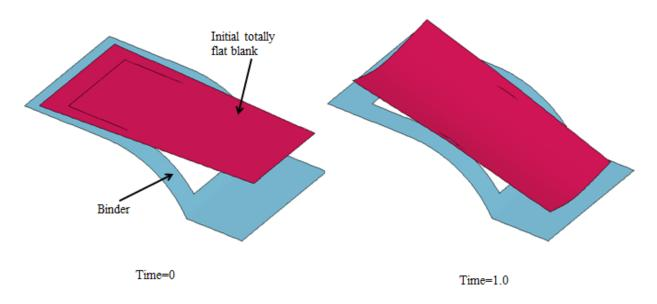
Figure 10. Switch from implicit dynamic to implicit static during gravity loading.
