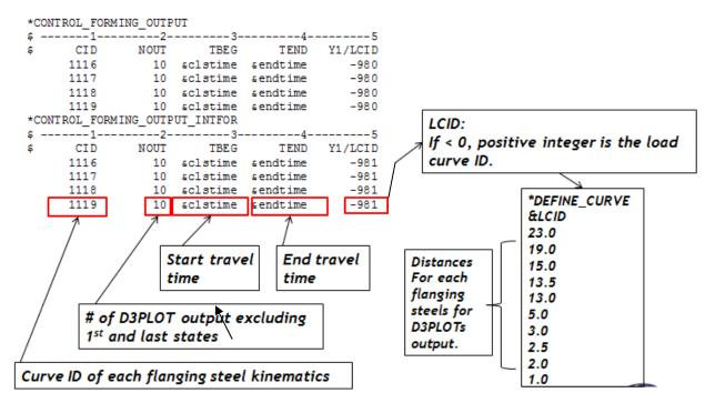
Figure 8. Output control for D3PLOT and INTFOR.
