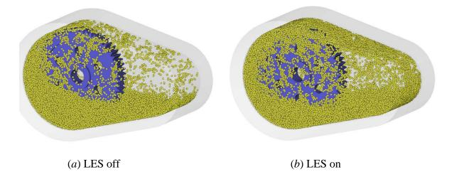
Fig.9 Gear oil flow simulation using MPS
