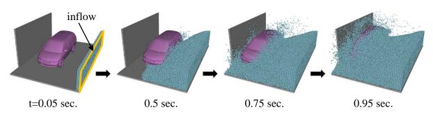
Fig.12 Result of tsunami simulation using MPS
