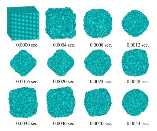
Fig.7 Shape change caused by CSF model of  $1mm \times 1mm \times 1mm$  water cube
