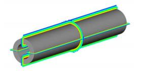
Fig.3 Wall distance function of a cylinder
