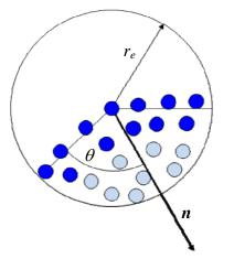
Fig.6 Surface tension model in MPS
