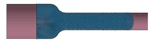
Fig.5 "push-in" analysis to simulate Newtonian viscous flow in SPH
