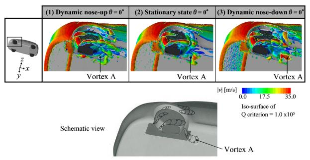
Fig. 14 Vortical structures in vicinity of Fr wheel house at pitch angle  $\theta = 0^{\circ}$  for different situations
