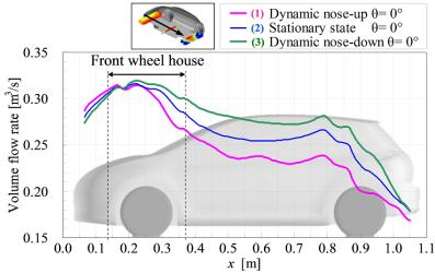
Fig. 12 Volume flow rate under model body at pitch angle  $\theta = 0^{\circ}$  for different situations
