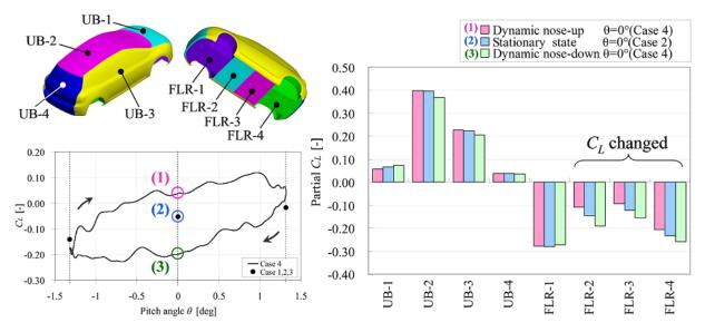
Fig. 8 Aerodynamic force  $C_L$  acting on each part of model body
