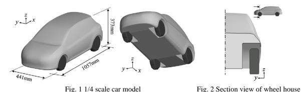
Table 1 shows the simulation cases. The simulation cases were made for three cases of stationary state and a pitching motion case. In all cases, mainstream velocity was 27.78 m/s, and the Reynolds number, which is based on the total length of the model, was  $Re = 1.91 \times 10^6$ . To represent the pitching motion, forced sinusoidal pitching oscillation was imposed on the body
