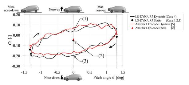
Fig. 7 Unsteady aerodynamic force during pitching motion and steady aerodynamic force
