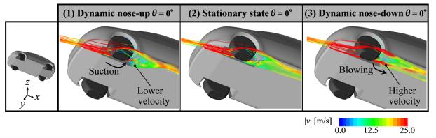
Fig. 13 Stream lines in vicinity of Fr wheel house at pitch angle  $\theta = 0^{\circ}$  for different situations
