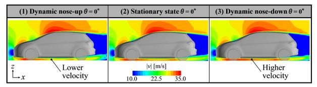
Fig. 11 Velocity magnitude distributions at y = 0 at pitch angle  $\theta = 0^{\circ}$  for different situations
