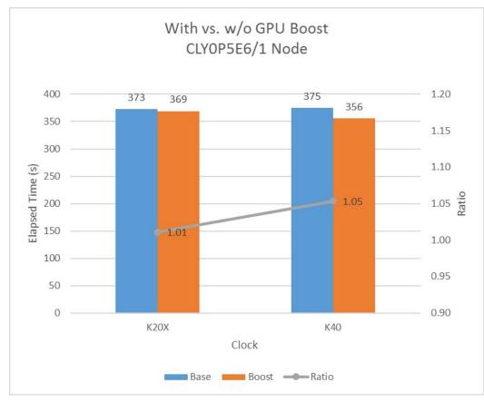
Figure 3 CYL0P5E6 elapsed times with and without GPU Boost
