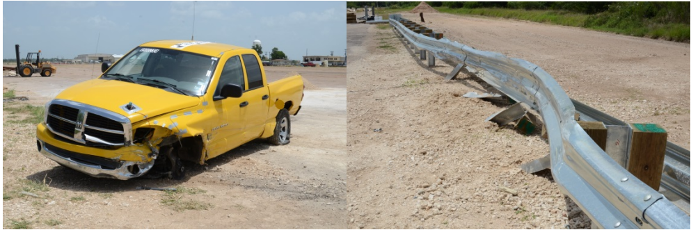
Figure 18 Vehicle and guardrail damage after MASH test 3-11
