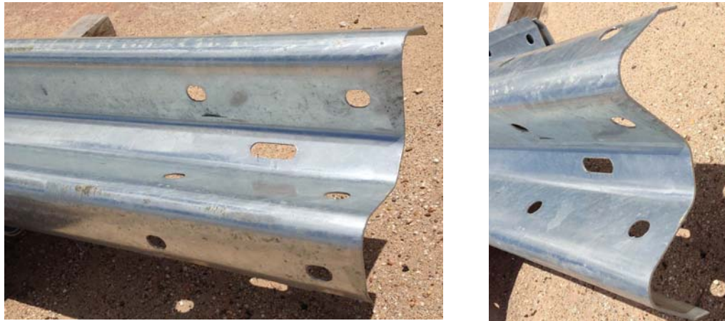
Figure 1 W-beam rail element showing the end (splice) section
