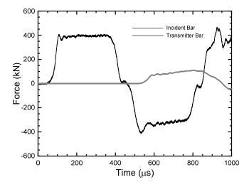
Figure 3: Waves recorded during a dynamic punch test with a hemisphirical punch.
