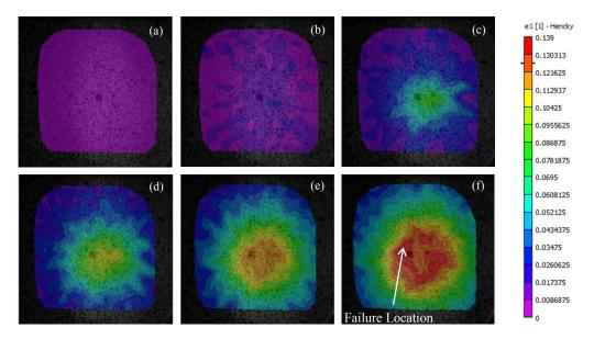
Figure 4: Maximum principal strain contours measured with 3D DIC: (a) 0µs, (b) 40µs, (c) 90µs, (d) 120µs, (e) 180µs, (f) 230µs
