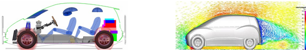
Figure 3: BEV packaging theme and aerodynamic study
